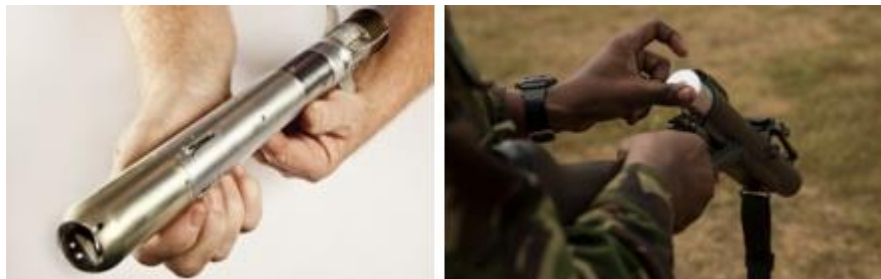
Raytheon's Pike is a 40 mm laser guided grenade round (left) can be fired from the older M79 (above right) or newer M320 launchers
